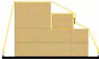
Isolate difficult to secure sections of the load regardless of shape.
