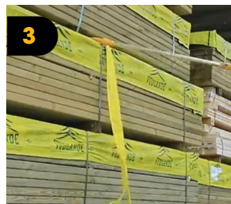
3 Thread a loop of the strap through the load using the ProPole
