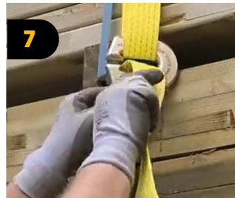
7 Loop the end of the tail strap over the load choker
