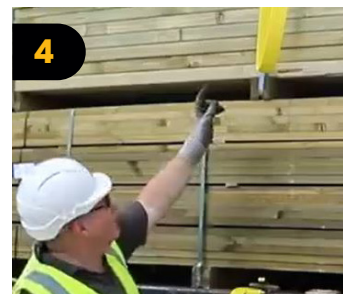
4 On the other side of the vehicle, pull down the webbing loop
