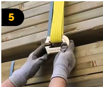
5 Attach the load choker to the webbing loop
